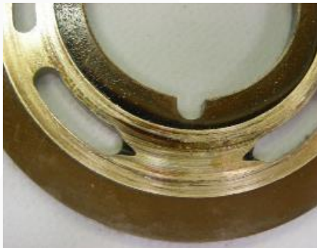
Some samples with excessive wear
